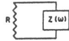
FIG. 3. A circuit with a resistance R and a block box of impedance Z(omega).
